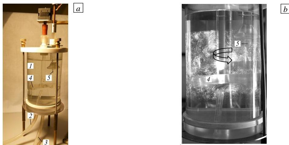
**Fig. 1.** Functioning continuous-flowing crystallizer (a): 1 – container; 2, 3 – tubes for solution inflow and outflow; 4 – mixer; 5 – crystal; (b) visualized flow structure during mixer reversed rotation at 1.57 rad/s.
