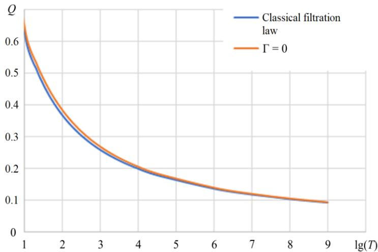
**Fig. 1.** For comparison of the production decline curves for classical filtration law and the filtration law with threshold pressure gradient at  $\Gamma = 0$ .
