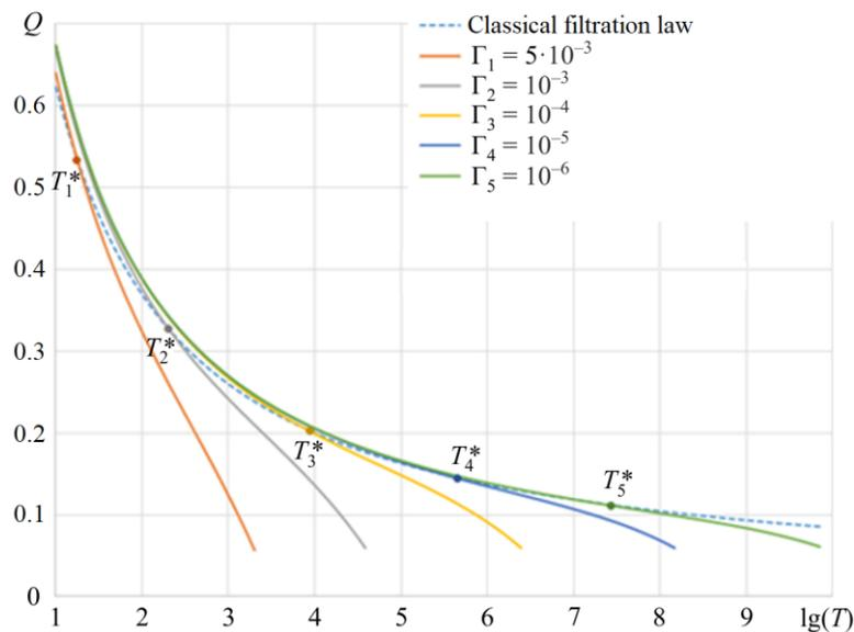
**Fig. 2.** Comparison of the production decline curves for the classical filtration law and the filtration law with threshold pressure gradient for different values of  $\Gamma$ .
