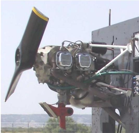
**Fig. 2.** Aircraft O-200 Engine.
