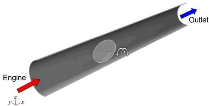
**Fig. 1.** Scheme of the noise reduction system with the flapper swinging inside the engine exhaust pipe.
