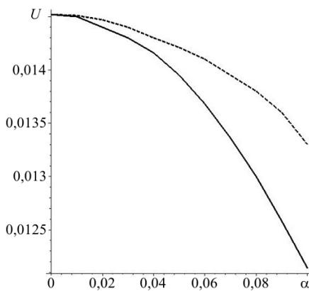
**Fig. 1.** Dependence of the radial displacement on the inner boundary of the cylinder on the gradient parameter  $\alpha$ ; exact (solid line) and approximate (dashed line).
