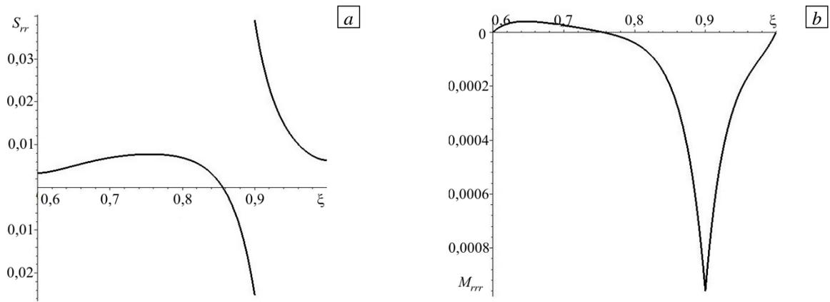
**Fig. 3.** Distribution along the radial coordinate  $\xi$  of the Cauchy radial stress (a) and couple stress  $M_{rrr}$  (b) at  $\alpha = 0,03$ .
