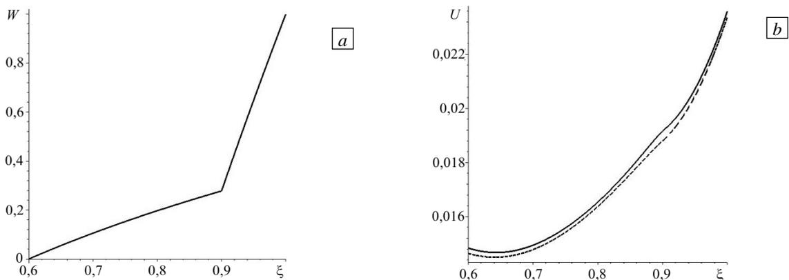
**Fig. 2.** Distribution along the radial coordinate  $\xi$  of temperature (a) and displacement (b); exact solution at  $\alpha = 0$  (solid line) and gradient solution at  $\alpha = 0,03$  (dashed line).
