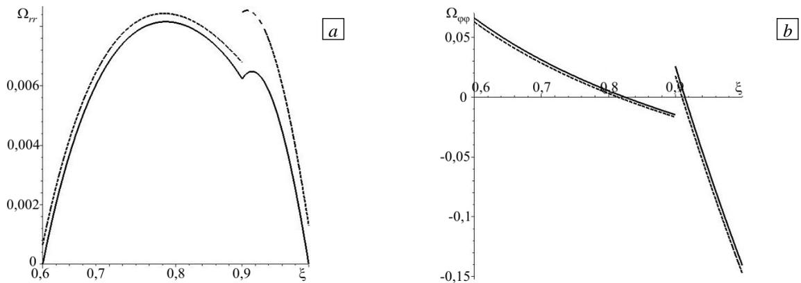
**Fig. 4.** Distribution along the radial coordinate  $\xi$  of total stresses: radial stress (a) and circumferential stress (b); exact solution at  $\alpha = 0$  (solid line) and approximate solution at  $\alpha = 0,03$  (dashed line).
