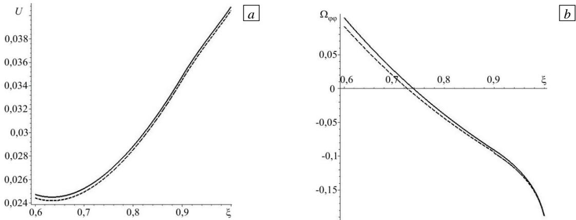
**Fig. 5.** Distribution along the radial coordinate  $\xi$  of displacement (a) and total circumferential stress (b); exact solution at  $\alpha = 0$  (solid line) and approximate solution at  $\alpha = 0,03$  (dashed line).
