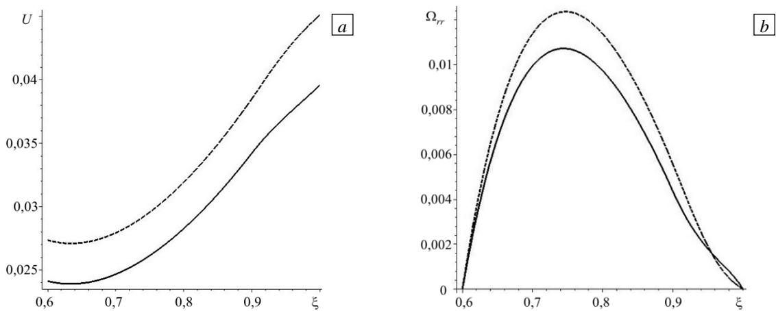
**Fig. 7.** Distribution along the radial coordinate  $\xi$  of the displacement (a) and the total radial stress (b) at  $\alpha = 0,03$  and different values of the inhomogeneity parameter  $N$  : 1 (solid line) and 2 (dashed line).
