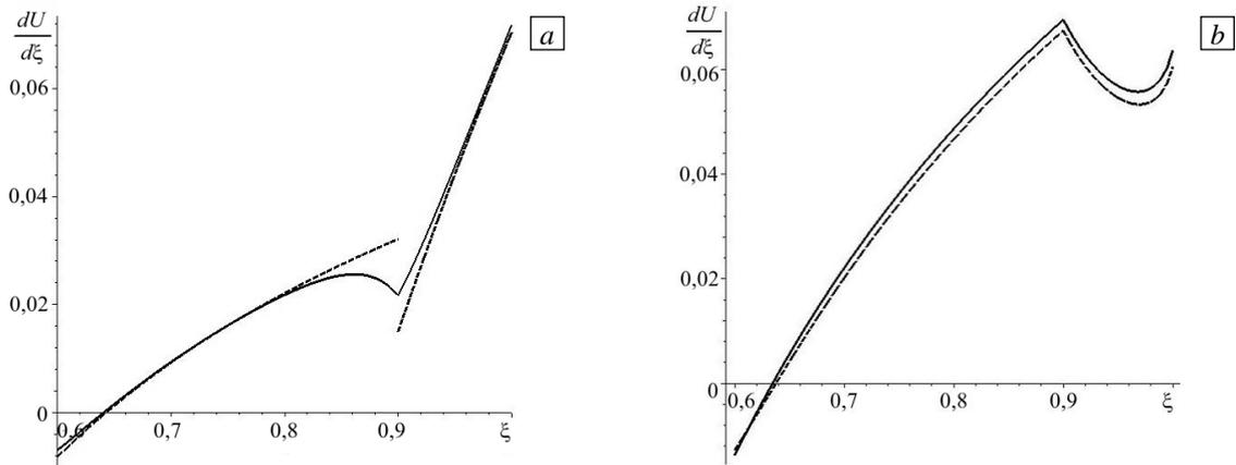
**Fig. 6.** Distribution along the radial coordinate  $\xi$  of deformations  $dU/d\xi$  in the cases of homogeneous (a) and inhomogeneous (b) coating; exact solution at  $\alpha = 0$  (solid line) and approximate solution at  $\alpha = 0,03$  (dashed line).
