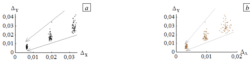
Fig.6. Change of \Delta_Y in relation to \Delta_X (a) and \Delta_A (b), determined in the series of experiment No 6; solid lines show the ranges of the results obtained; as the norms of deviation of influences and operator parameters decrease, the norm of deviation of the response from that obtained during the base calculation also decreases.
