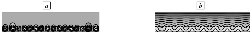
Fig. 5. Isolines of the stream function (a) and the concentration distribution of the first component of the mixture (b) at the time instant t = 1 at \gamma = 1/50 .
